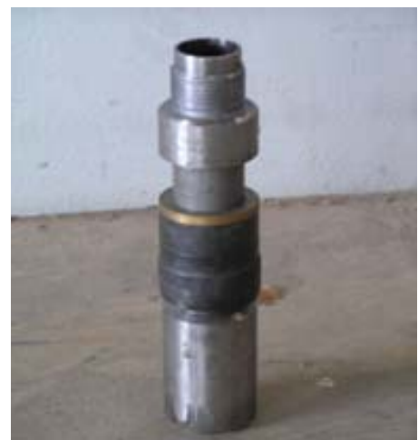
Example of sealing element for Tubing Isolation Tool
