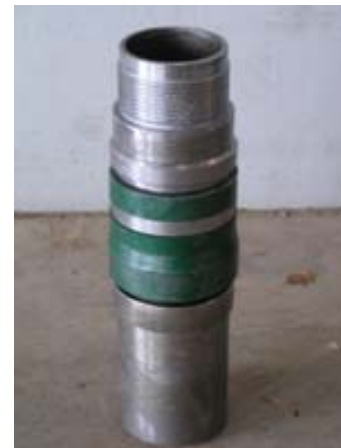
Example of sealing element for Casing Isolation Tool
